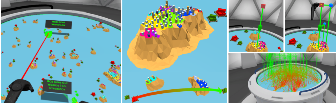
Figure 1: The software visualization application IslandViz for OSGi-based systems in virtual reality. (left) Software modules are represented as islands. (middle) Islands have very distinct shapes. Dependencies between them are visualized with arced arrows. (right top) Service connections are routed via nodes and distributed over the available height. (right bottom) All service and bundle dependencies of a complex software system are shown simultaneously inside the bounds of a virtual table.
