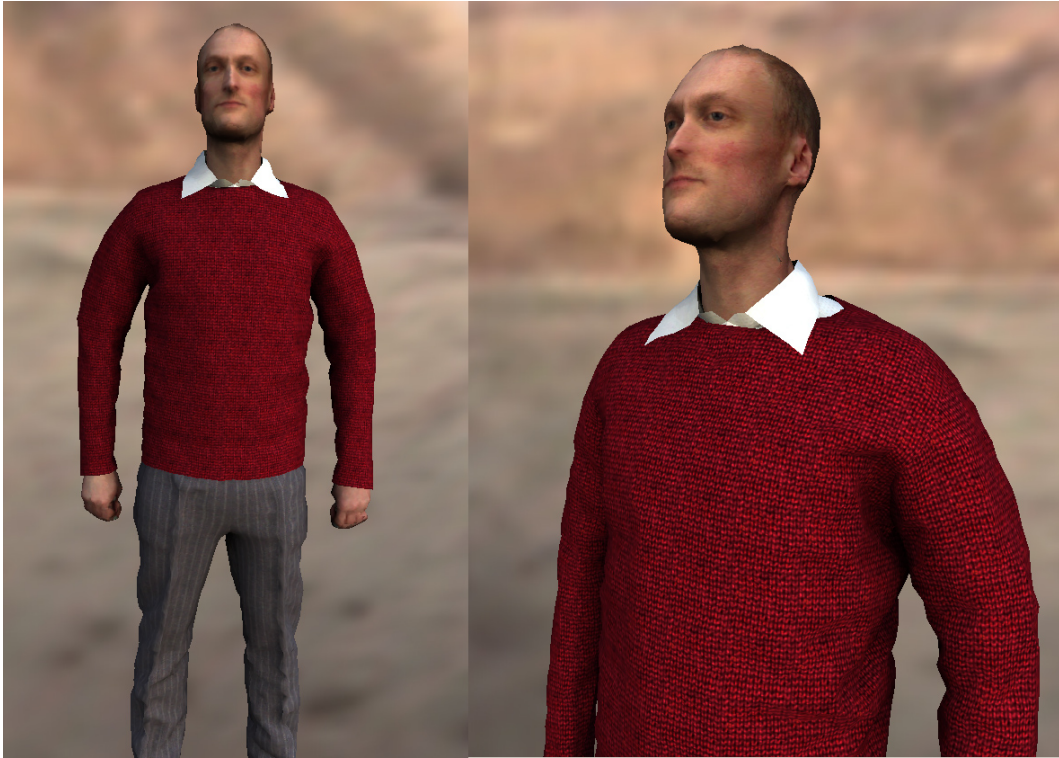
Figure 6: An example of four layers of garments: A shirt, trousers, a pullover and the collar of the shirt. Although the shirt is dressed at first, its collar has the property of being on top and hence it lies above the pullover.
