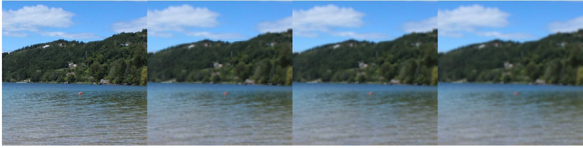
Figure 1: Comparison between different upscaling techniques. The original is rendered in 1000x1000 pixels, the other images are upscaled from 125x125. From left to right: Full render, Nearest Neighbor, Bilinear Interpolation and Bicubic Interpolation.
